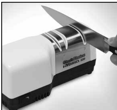
Figure 4. Knife in Stage 2. Use back and forth sharpening strokes with modest downward pressure. See text.
