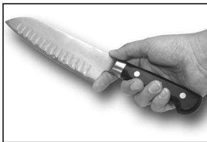
Figure 12. If your blade has a significant choil it may be helpful to place our finger behind it as shown when sharpening.
