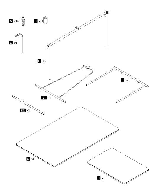
Connect parts **D** & **E1** & **E2** and position up-side-down on the bottom side of the tabletop **G**. **Pay close attention to the orientation of the holes on the part E2 before mounting!**
