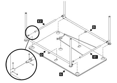
Force parts **F** into the longitudinal tubes of the part **D** until fully closed. Expect 3 distinctive "clicks" along the way.
