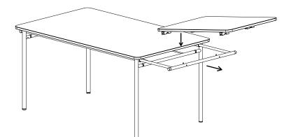
With fully extended parts 🖪 lower the side tabletops 🖪 rotated lonigitudinally onto the supports of the parts 🖪 .
