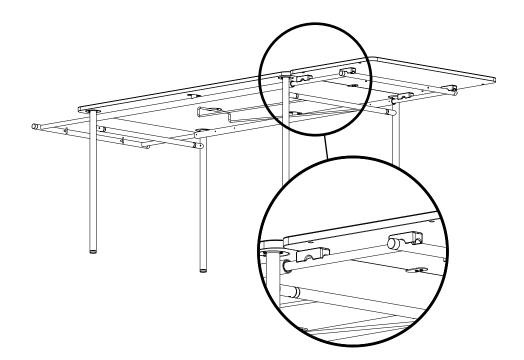
Rotate side tabletops **H** for 90° with plastic spacers facing the table. Position side tabletops **H** on the fully extended parts **E**.
