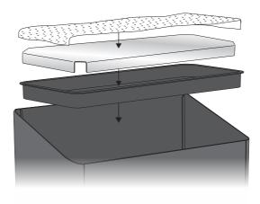
3. To install the glass, carefully guide the C-shaped opening through the S-shaped metal bracket inside the planter. Gently lower the glass from the top until it rests securely on the metal ledge inside. Ensure the glass sits on the metal ledge and not on the edge of the planter box.
